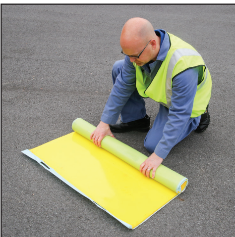
Step 5. When the cover is completely clean of dirt, debris and spill residue, be sure the polyurethane side is up and roll the cover onto its silicone fabric.
